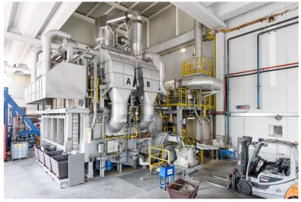
A Hertwich state-of-the-art Ecomelt-PR multi-chamber melting furnace for ecological and economic melting of loose scrap with moderate organic content (reference plant of similar design)
